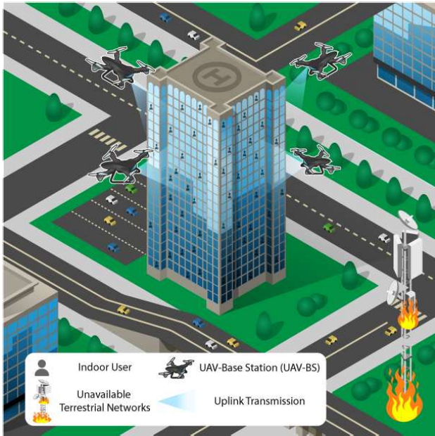
Fig. 1. UAV-BSs emergency indoor user service network.
